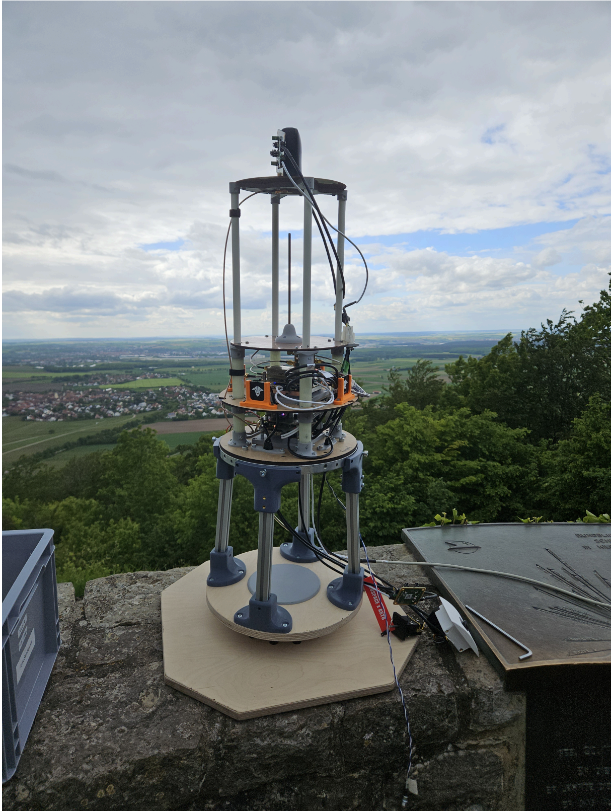
Figure 1: Full avionics stackup during a range test
